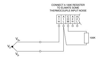
Figure 4-28. Thermocouple Wiring
